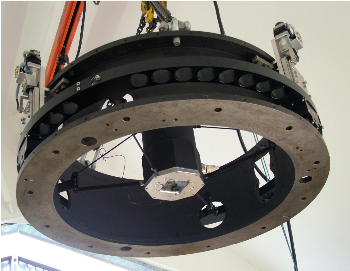
Fig. 5. Telescope tube with the dewar mounted, spider vanes passing through the existing holes in the telescope tube.
