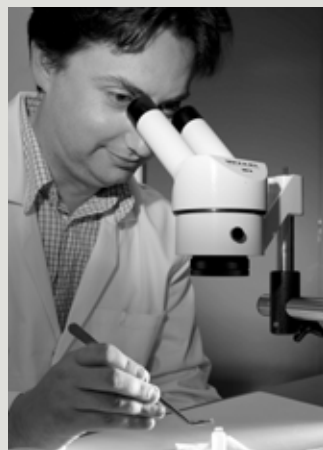
Above: AAO staff member Anthony Horton assembling a micro-lens array for CYCLOPS. Photo: Tim Wheeler
