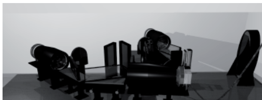
Figure 2.1 A design model of the HERMES spectrograph (Image: Andrew McGrath)
