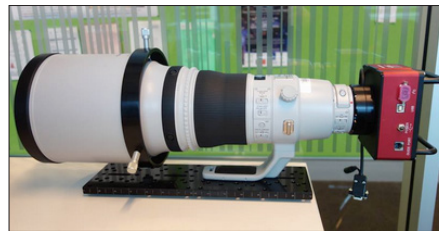
Figure 2 The Huntsman Telephoto Eye – Canon EF 400mm f/2.8 L IS II USM lens, coupled to a science-grade commercial SBIG STM-8300m CCD camera using a Birger Canon EF-232 adaptor.
