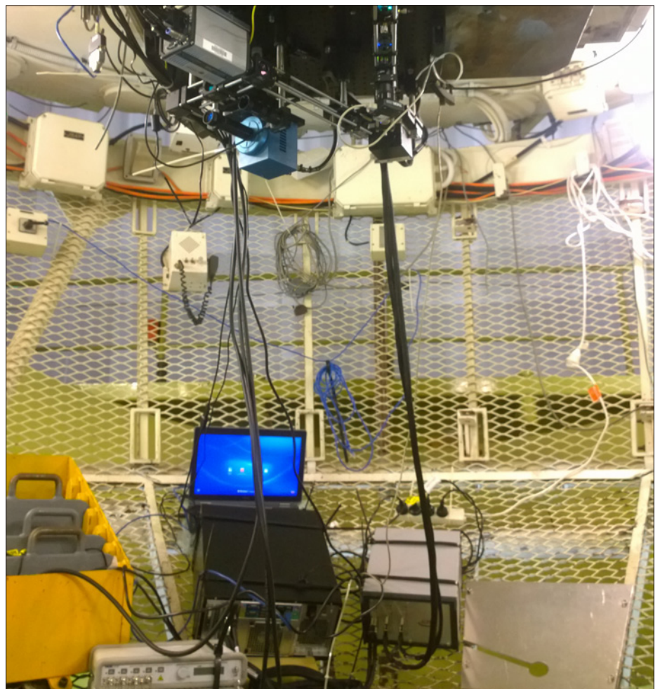
Figure 1: Photo of the adaptive optics test-bed mounted on the Cassegrain focus on the AAT.
