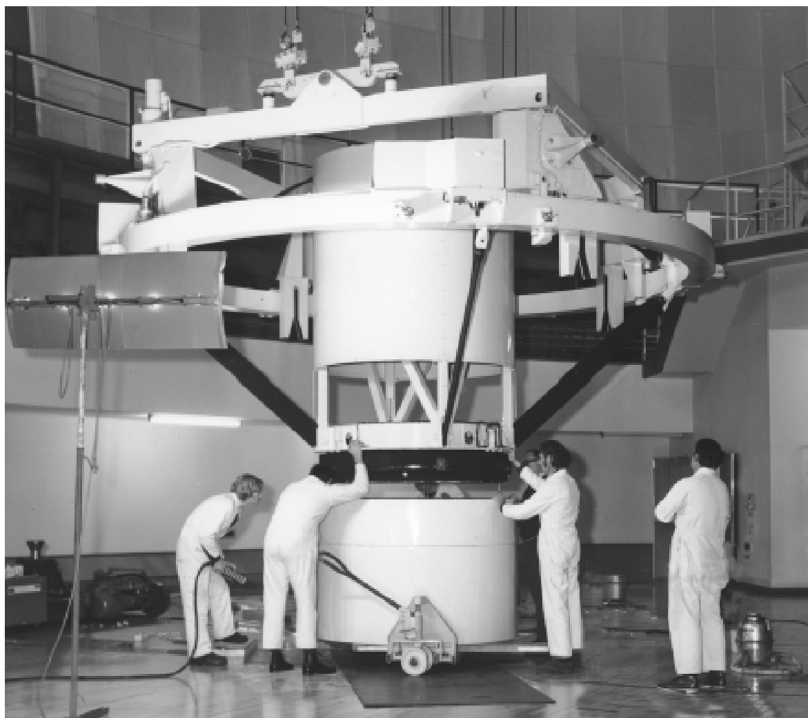
On 27/4/99 staff at Siding Springs celebrated the Twenty-fifth Anniversary of first light at the AAT. In this issue we look back to those early commissioning days (page 7). Here we see the commissioning team putting the f/8 top end together.
